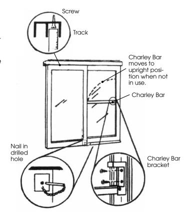
drilled hole will prevent opening. For fire safety, never put a pin at the top of the window. Be aware that as sliding door frames wear over time, holes may not line up and pins may no longer fit.
