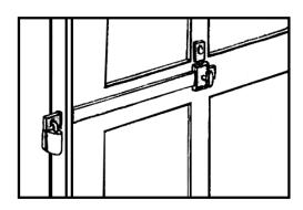
Double garage doors that are side-hinged can be made more secure by installing cane bolts.
