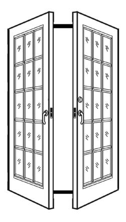
Double doors of any kind should have one door braced with a recessed cane bolt (check your hardware store). When the bolt is pushed down, it leaves only one door active. Install a deadbolt lock in the other door.
